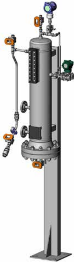
Fig. 23 API Plan 52 Seal Pot Assembly Assembly shown with some optional components.
